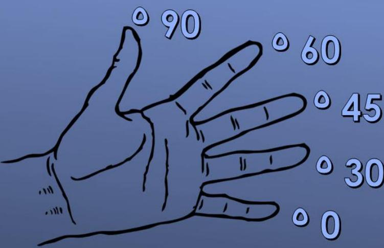
Diagram illustrating the relationship between the number of fingers held up and the corresponding angle in degrees:
